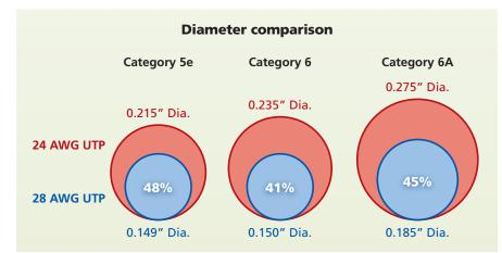
Drawn to proportion, these illustrations show the difference in outside diameter of Category 5e, 6, and 6A cables containing 24-AWG conductors (red) and those containing 28-AWG conductors (blue). In all cases, 28-AWG cables are less than half the size of 24-AWG cables.
