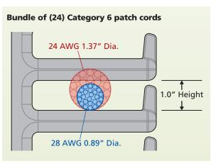
A bundle of 24 Category 6 patch cords with 24-AWG conductors is too large to fit through the 1-inch finger opening of vertical cable managers, while a bundle of 24 Cat 6 cords with 28-AWG conductors easily fits through the opening.
