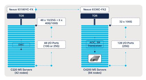
Figure 3. Rack density optimization using multimode chassis
