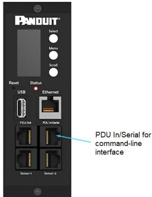
**Figure 21: Connect the RJ-45 end of the cable to the PDU In/Serial connector**
