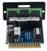
Figure 14: Relay Card Front and Top View (showing connection points)
