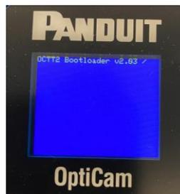
*Image of the bootloader screen, indicating the tool is ready to accept the firmware update. **This screen will time out after 60 seconds if the update process is not initiated.** The user may have to restart the process from the Settings menu.*
