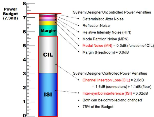
**Figure 3. Optical channel budget for 10 Gb/s Ethernet (10GBASE-SR).**
