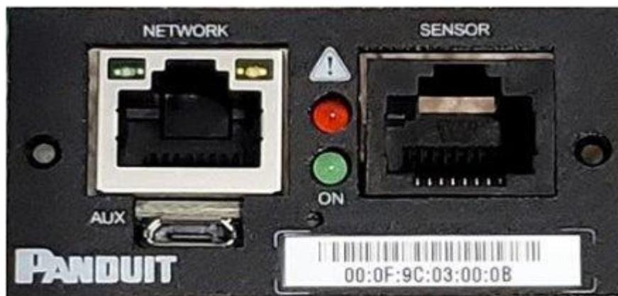
**Figure 1: Ethernet Port for Network Connection**
