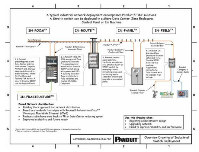
A plant network layout using zone architecture reduces cabling installation, localizes network traffic to improve network resiliency, improves capability for network redundancy and reduces cost of future expansion. To learn more about this zone cabling system, visit http://goo.gl/6NSUwV.
